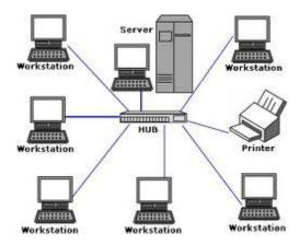
The connections can be cable, fibre-optic, or wireless (infra-red, microwave or radio).
